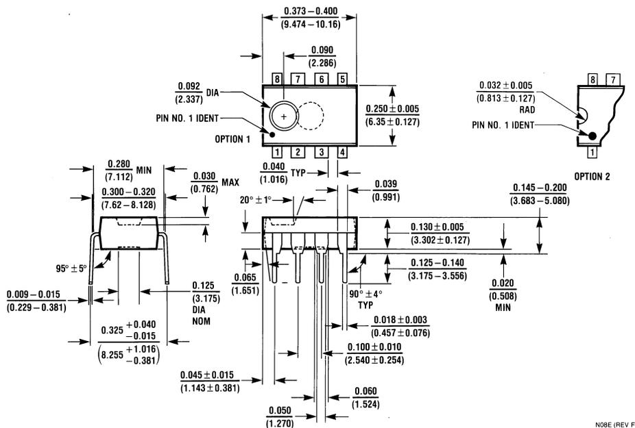
**8-Lead (0.300" Wide) Molded Dual-In-Line Package**
